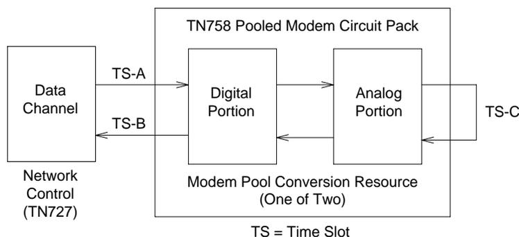
Figure 5-42. Modem Pool Conversion Resource Loop Around Test Set-up
