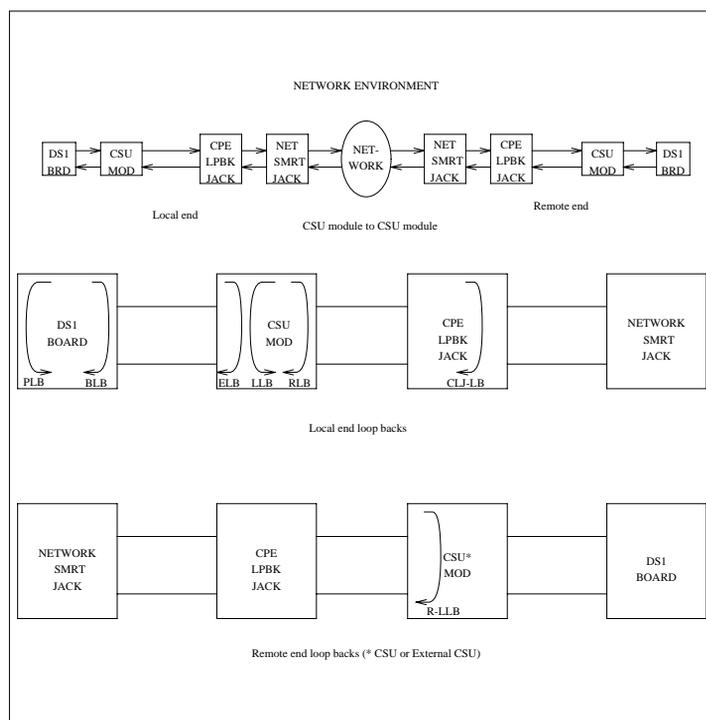
Figure 5-21. High Level Overview Of Loopback Points
