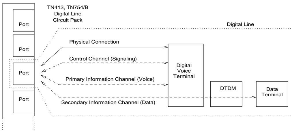
Figure 5-19. Digital Line Connectivity
