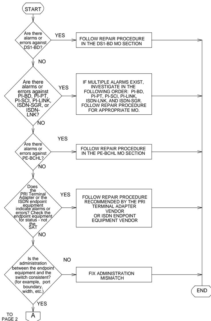
Figure 2-8. Processing of PRI endpoint problems (page 1 of 2)
