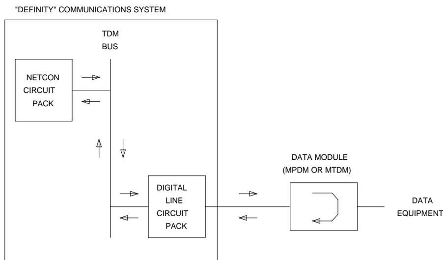
Figure 5-47. Internal Loop Around Test
