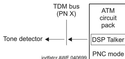
Figure 5-10. ATM Cross Talk Test #1298 schematic
