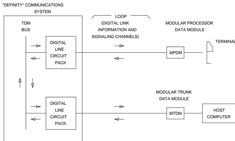
**Figure 5-46. Typical Data Module Application**
