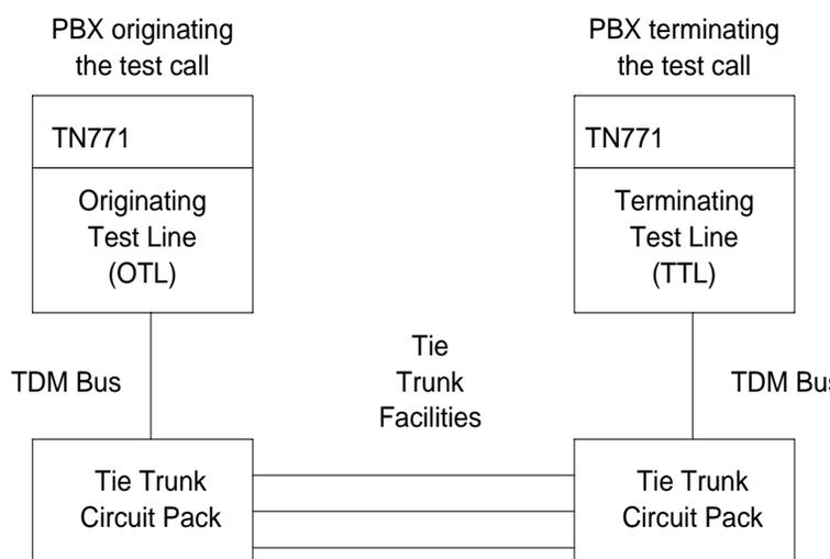
Figure 5-43. ATMS Tie Trunk Test Call
