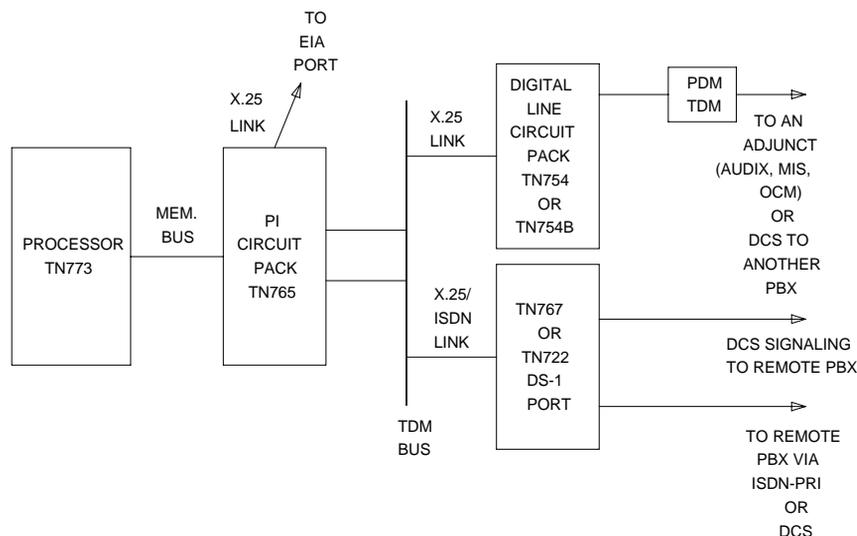
Figure 5-50. Processor Interface Link Interactions
