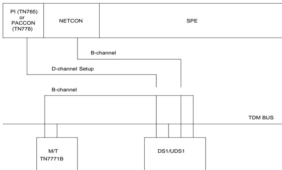
Figure 5-30. ISDN-PRI Outgoing Test Call
