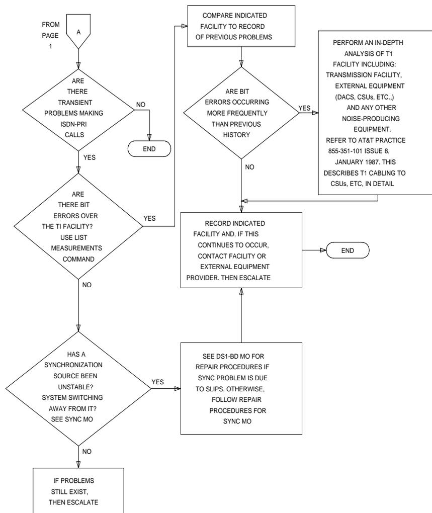
Figure 2-7. Processing of ISDN-PRI problems (page 2 of 2)
