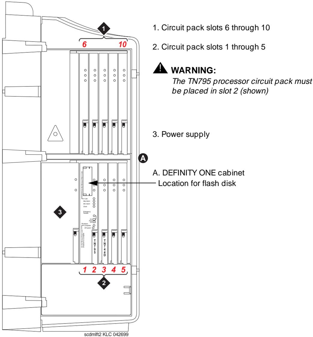
Figure 1-1. Compact Modular Cabinet (CMC) slot configuration
