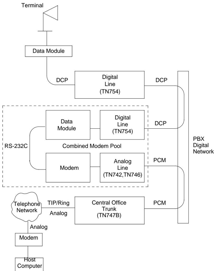
Figure 5-41. Typical Modem Pool Switched Connection with Combined Modem Pool
