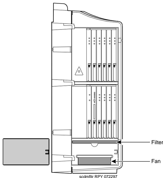
Figure 2-1. Fan/filter removal
