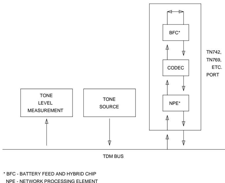
Figure 5-3. Analog Loop Around and Conference Test
