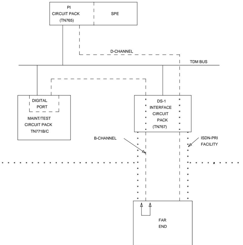
Figure 5-44. ISDN-PRI Outgoing Test Call
