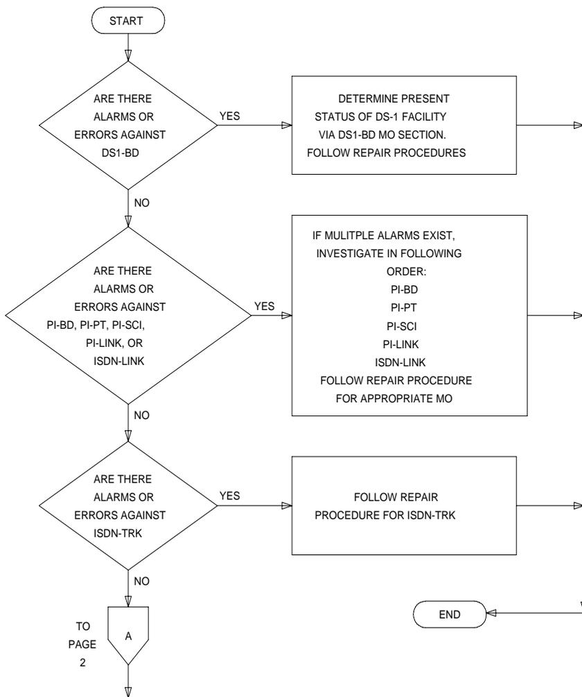
**Figure 2-6. Processing of ISDN-PRI problems (page 1 of 2)**
