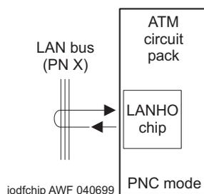
**Figure 5-7. Packet Interface Test (#598)**
