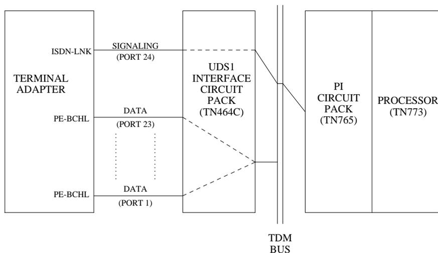
Figure 5-48. PRI Endpoint Port Interactions [INTEL]
