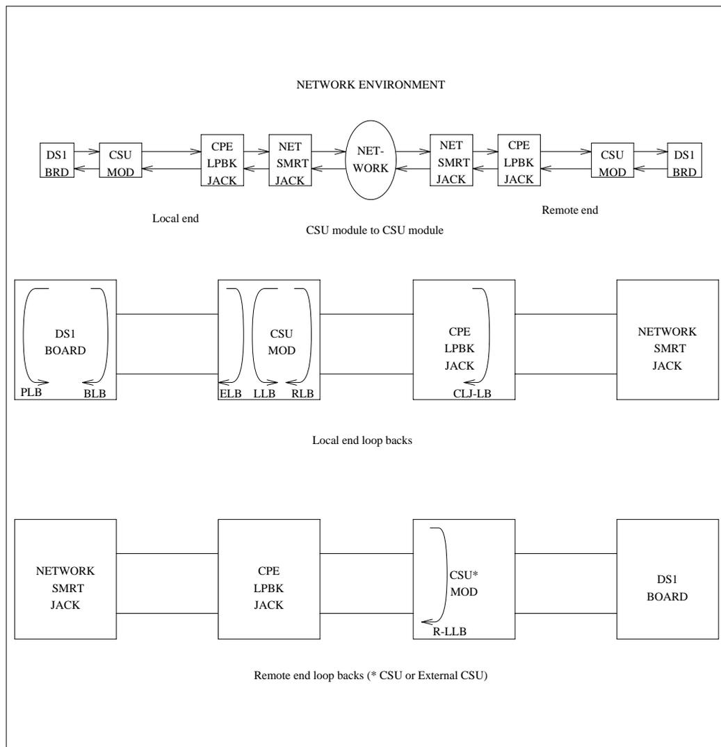
Figure 5-55. High Level Overview Of Loopback Points
