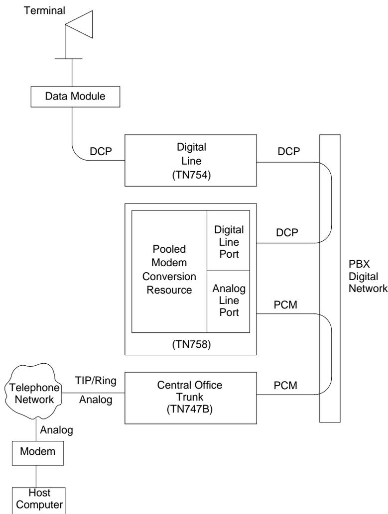
Figure 5-40. Typical Modem Pool Switched Connection with Integrated Pooled Modem
