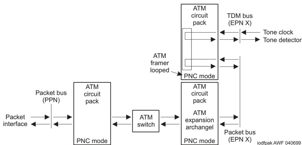
**Figure 5-9. ATM Board Framer Looparound Test (#1260)
